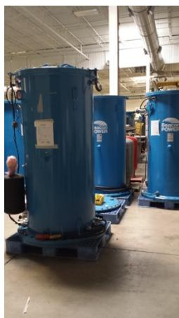
Figure 4 - FES rotor package
